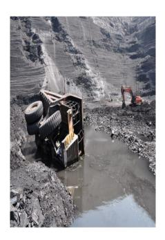
Prima facie cause of the accident: While a dumper was being driven in night shift of an opencast coal mine, it accidentally toppled into a sump of 2 m deep adjacent to the coal face, the operator, sitting in the cabin drowned and succumbed almost instantly.
